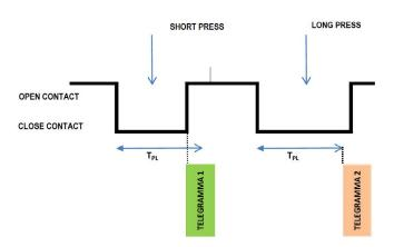
When the input is closed, the time count starts; if the input is opened before the time exceeds the time TPL, the device executes the command associated with the "short closure" event and if, instead, the timeout TPL expires and the input is still being closed, the command associated with the "long closure" event is executed.
