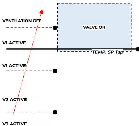
The shaded area represents the temperature range defined by the "heating control differential ON" parameter in case of increasing temperature. When the temperature decreases, the "heating control differential ON" parameter defines the valve hysteresis.
