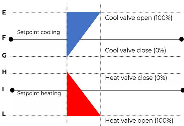
This makes it possible to adjust the opening and closing of the additional valve independently of the speed control (for example, once the setpoint has been exceeded, a maintenance action can be taken keeping the valve open again without activating the speeds).
